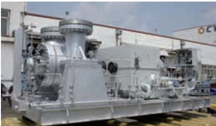
SPEC : 3739.8m 3 /hr x 88.7m x 1200kW (Turbine)
