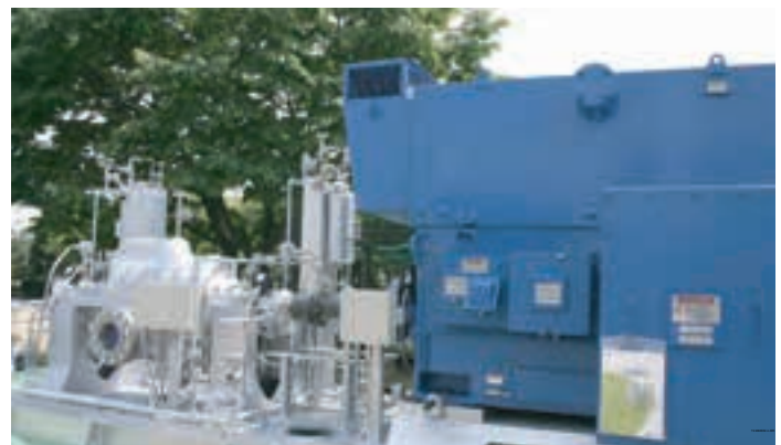
SPEC : 309.6m 3 /hr x 505m x 650kW (2Pole)
