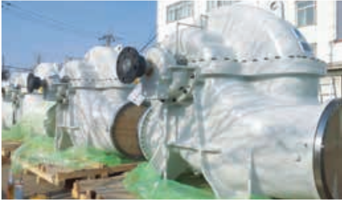
SPEC : 18000 m 3 /hr x 48 m x 3000 kW x 590rpm
